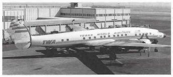
At first, Lockheed proposed the model 1549 with Allison 501 turboprops, but ultimately, 3,400 hp turbo-compound Wright 3350 EA-2 engines were chosen for what would become the model 1649A. Larger, 16-ft, 10-in diameter propellers were incorporated as well.
